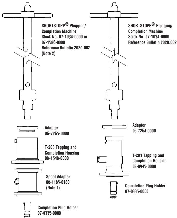
■ Note 1: 12-inch Spool Adapter required to set 12-inch SHORTPLUG™ with Guide Bars in SHORTSTOPP Type II 3-Way™ Tee fittings using the 06-1546-0000 Adapter and 07-1586-0000 Completion Machine
