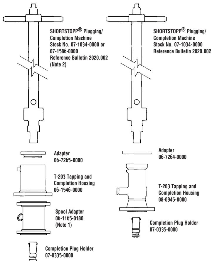
■ Note 1: 12-inch Spool Adapter required to set 10-inch SHORTPLUG™ with Guide Bars in SHORTSTOPP Type II 3-Way™ Tee fittings using the 06-1546-0000 Adapter and 07-1586-0000 Completion Machine
