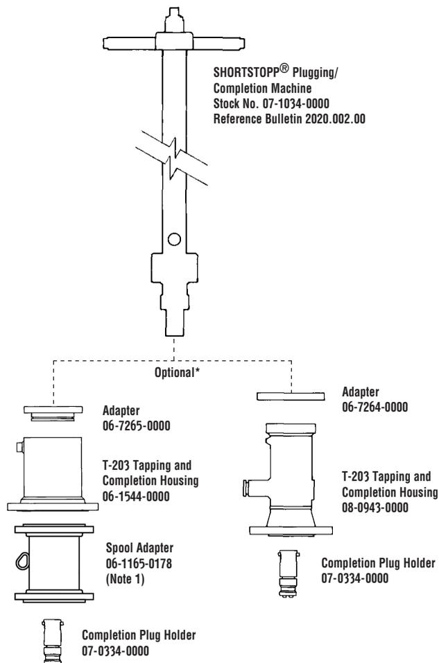
■ Note 1: 8-inch Spool Adapter required to set 8-inch **SHORTPLUG™** with Guide Bars in **SHORTSTOPP** Type II 3-Way™ Tee fittings using the 06-1544-0000 Adapter.
