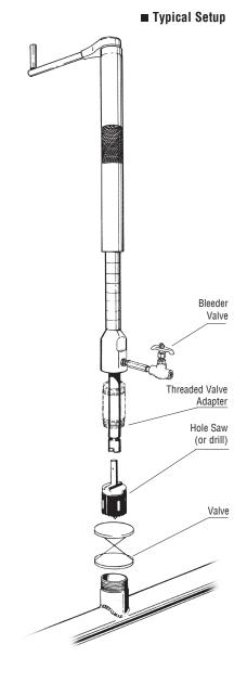
\* The 904 Drilling Machine is a higher pressure (balanced) version of the T101B XL machine. It is rated at 2,220 psi (150 bar) at 180°F (82°C). For special requirements, such as higher pressure or temperature, consult the factory.
