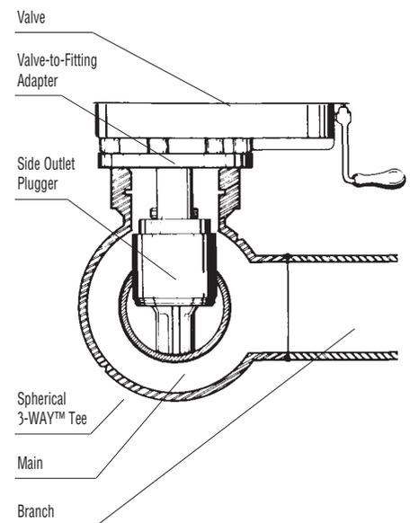
The SHORTSTOPP® 275 system's Side Outlet Plugging Machine is used with Spherical 3-WAY™ Tees to plug the tapped hole in a main. It forms a pressure-tight seal that simultaneously allows flow to continue in the main while preventing it from escaping into the side outlet. This permits maintenance work on the branch line without interruption of flow in the main line.
