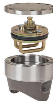
■ 4- to 12-inch Welding fitting includes cover flanges with bolts, gasket and plastic caplugs, SHORTPLUG™ with Guide Bars, O-ring and flanged nipple.
