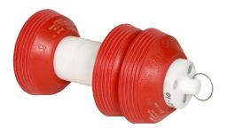
3C configurations are recommended for light cleaning, line filling and dewatering, batch separation and liquid removal. They are normally used in pipelines up to 100 miles (161 km) in length. (For longer runs, a 4C configuration would be recommended. For operating pipelines, a 4C or DCDC configuration is recommended.)
