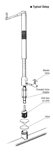
\* The 904 Drilling Machine is a higher pressure (balanced) version of the T1018 XL machine. It is rated at 2,220 psi (150 bar) at 180°F (82°C). For special requirements, such as higher pressure or temperature, consult the factory.
