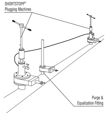
TDW SHORTSTOPP® Purge & Equalization Fittings are used for blowdown of the isolated pipe section following a double SHORTSTOPP® operation.
