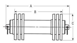
6D configurations are recommended for bi-directional applications in which the pig has to be run in two directions before being removed from the line. They are normally used for line filling-testing-dewatering applications in lines up to 60 miles (97 km) in length.
