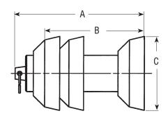
3C configurations are recommended for light cleaning, line filling and dewatering, batch separation and liquid removal. They are normally used in pipelines up to 100 miles (161 km) in length. (For longer runs, a 4C configuration would be recommended. For operating pipelines, a 4C or DCDC configuration is recommended.)
