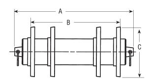
4D configurations are recommended for bi-directional applications in which the pig has to be run in two directions before being removed from the line. They are normally used for line filling-testing-dewatering applications in lines up to 40 miles (65 km) in length.
