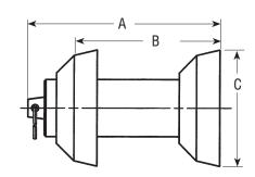
2C configurations are recommended for light cleaning, line filling and dewatering, batch separation, and liquid removal. They are normally used in pipelines up to 50 miles (80 km) in length. (For longer runs, a 3C or 4C configuration would be recommended. For operating pipelines, a 4C or DCDC is recommended.)
