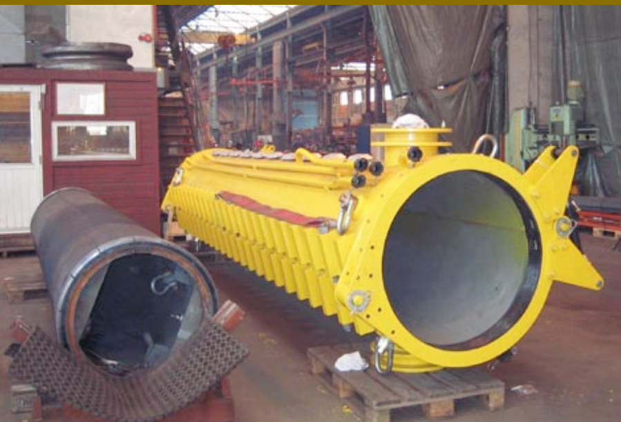
Grouted riser clamps for repair in the splash zone.
