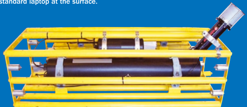
The typical communication range for the subsea communication unit is 2 km (1.2 M/6560 ft)
