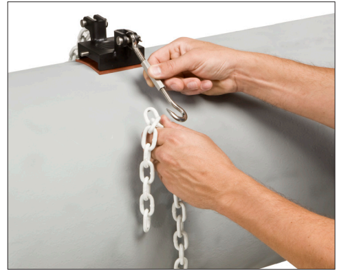
■ 2. Wrap chain around pipe and connect using hook on end of turnbuckle.
