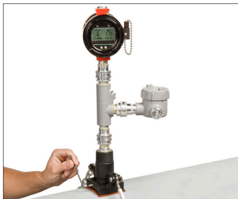
■ 5. Tighten set screw in base.
