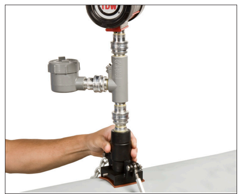
■ 4. Thread device (unit) assembly into base.
