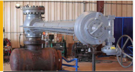
Double-Hub Assembly to perform the pressure test.
