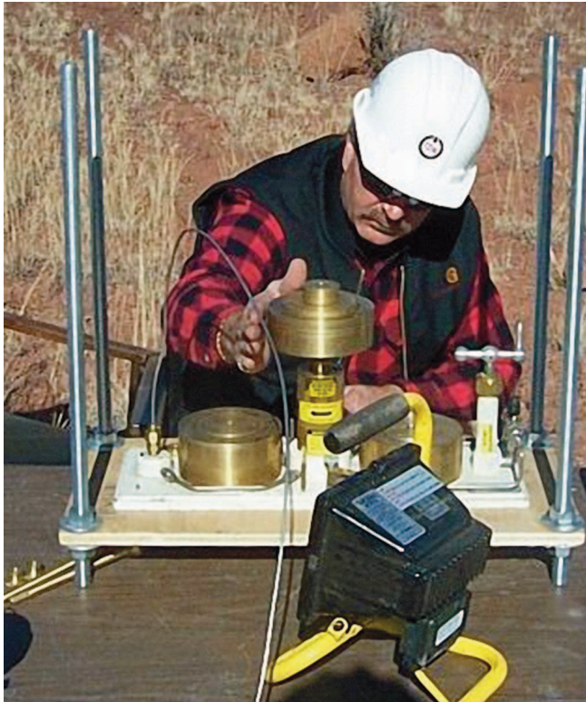
Figure 4. A variety of instrumentation, including dead weights, may be used to gauge pressure levels in the line during hydrotesting.
