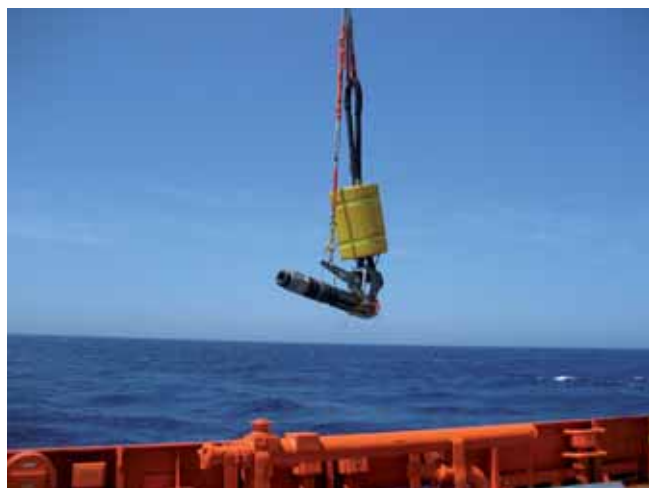
Figure 5. The custom SmartLift™ PRT is deployed from the lay vessel.
