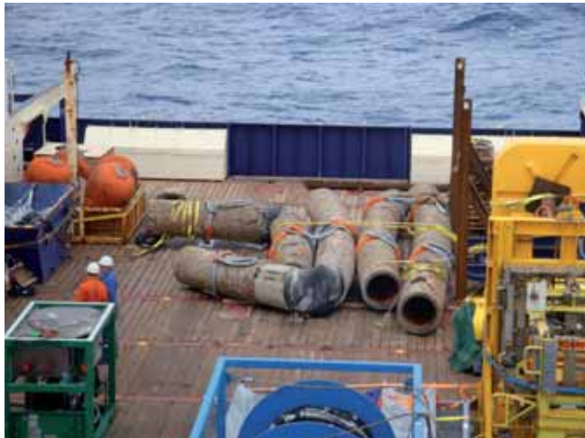
Figure 2. When a 26 in. pipeline was completely severed by a dragging anchor, it resulted in catastrophic failure of the line. The recovered pipe was severely deformed.
