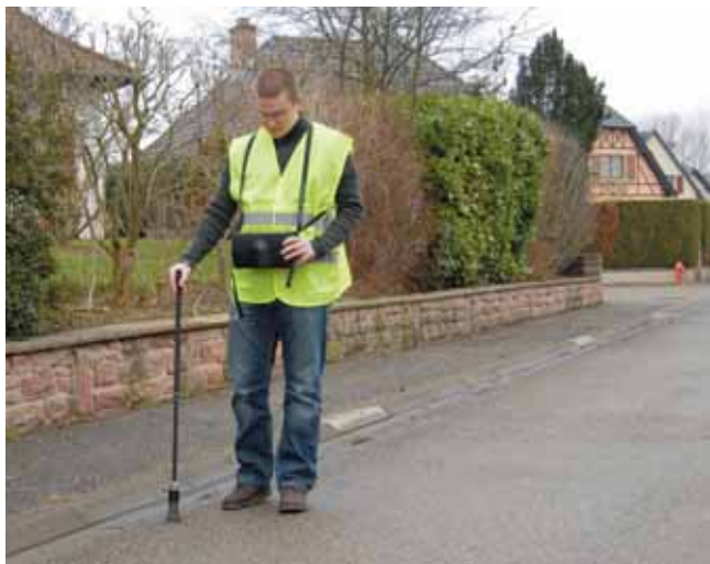
Figure 1. Foot surveys using portable laser detectors offer high precision but can be manpower-intensive and time consuming.
