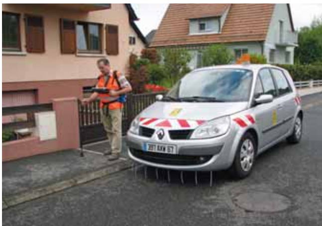
Figure 2. Leak survey and detection is usually accomplished using a road-driven vehicle. A vehicle survey offers the ability to quickly cover large areas, but not all areas are accessible to vehicles. A combination vehicle-foot survey is often employed.
