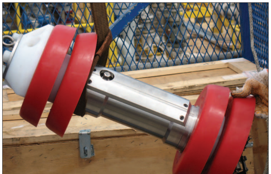
T.D. Williamson’s Semi-Smart V-Jet Pig just prior to an offshore run in Southeast Asia.
