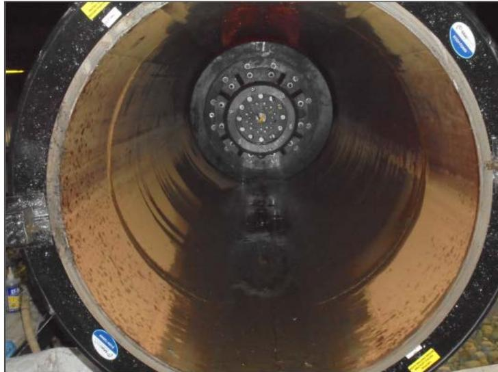
**SmartPlug™ tool isolating pipeline section at 16 bar (232 psi)**
