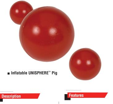
UNISPHERE<sup>™</sup> Pigs are seamless, liquid-cast polyurethane spheres. They are designed for heavy-duty service in the removal of liquid hydrocarbons and water from pipelines and piping systems. UNISPHERE Pigs are undersized and can be sized to match most any pipe ID. The inflating valve(s) on the UNISPHERE Pig may be used for inflating or deflating purposes.
