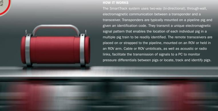
The accurate, reliable and cost-saving SmartTrack™ system revolutionizes pig tracking by using remote, two-way, through-wall electromagnetic communication between a transponder and transceiver.
